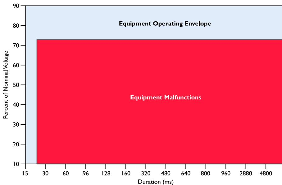
Figure 2: Dip-Tolerance Curve of a Sensitive PLC
