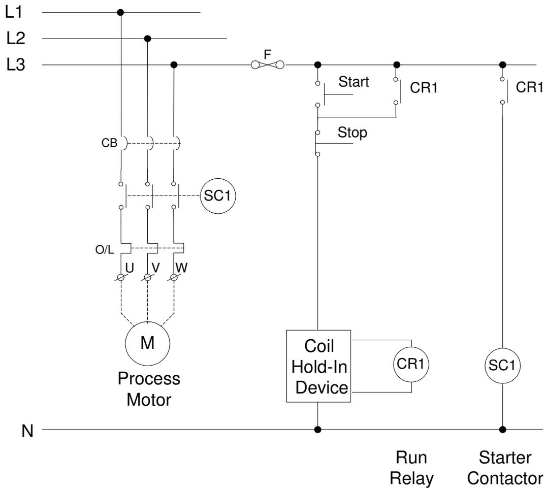
Figure 7: Relay or Contactor Circuit with Coil Hold-In Solution
