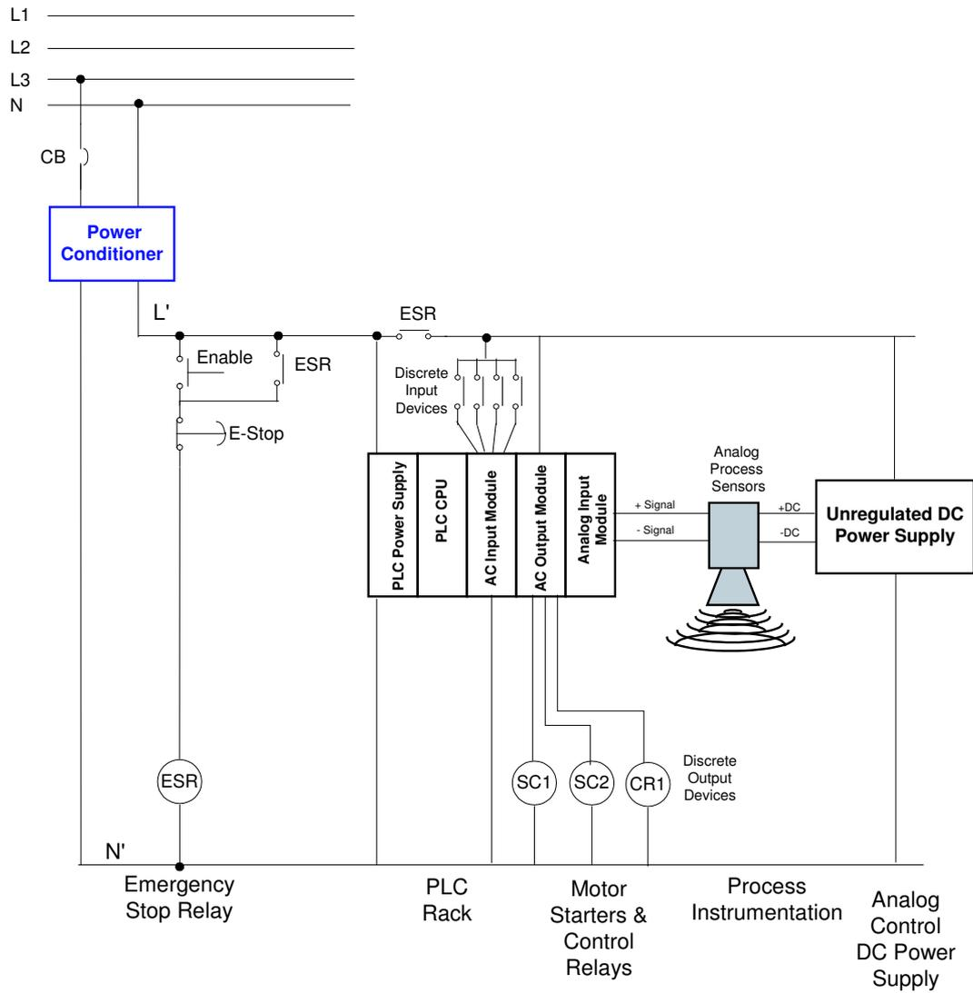
Figure 11: Common Power Source Power Conditioning Solution
