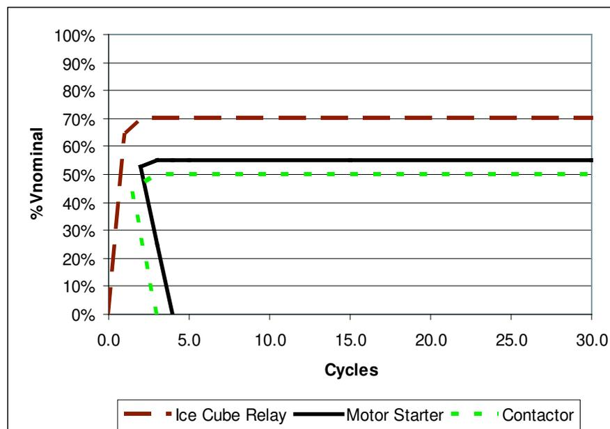
Figure 6: Example Dip-Tolerance Curves for Relays, Contactors, and Motor Starters
