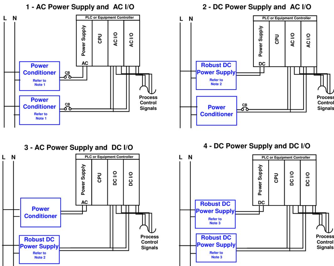
Figure 10: PLC Voltage Dip Hardening Solutions [8]
