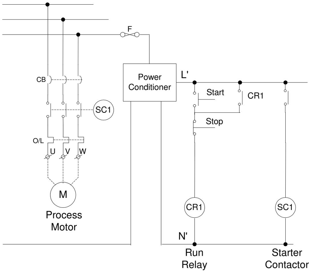
Figure 8: Relay or Contactor Circuit with Power Conditioner Solution
