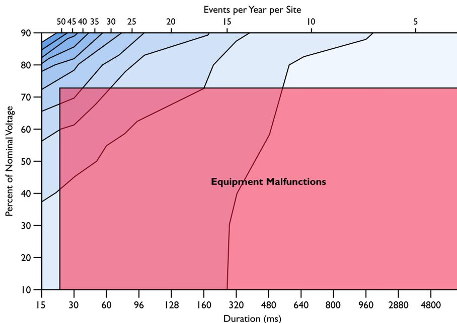
Figure 3: Dip-Tolerance Curve Imposed on the Voltage-Dip Contour Chart
