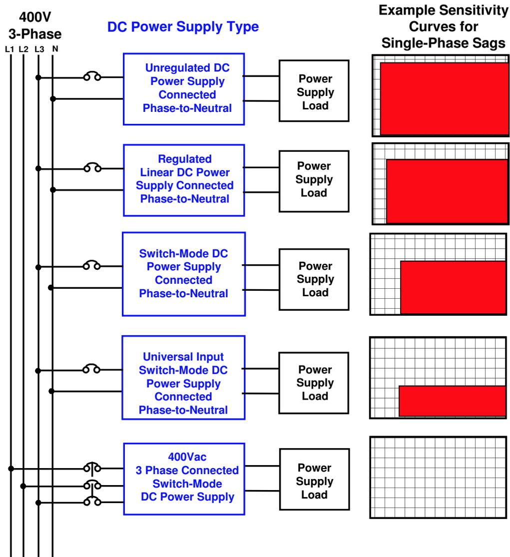
Figure 9: DC Power Supply Selection - With Respect to Voltage Dip Response, Worst (Top) to the Best (Bottom)
